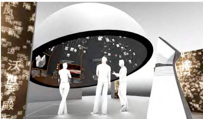
12m 360° dome projection system with 8 multimedia terminals and multi-layered animation, multimedia content and realtime information
