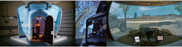
simulator is the most powerful in the entire automotive industry. With this driving simulator, highly dynamic driving manoeuvres such as changing lane can be simulated in a realistic manner, enabling in-depth research into driver and vehicle behaviour on the road. At the Driving Simulation Center of Daimler AG all Simulators (MBS-, Ride-, Fixed-Base-, Assistance Systems Simulator etc.) are housed under the one roof.
